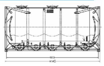
Dimension : Length x Width x Height: 6058 x 2495 x 2896 mm
